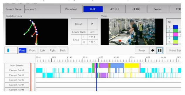
Toyota Motors Europe's JT/SJT system incorporates Xsens motion capture technology to monitor the physical health of its staff and maintain a safe, efficient workplace. The data captured by MVN Analyze<sup>™</sup> provides an accurate understanding of workers' posture during the build cycle. It is then used for posture awareness training and to implement design changes on processes and vehicles.
